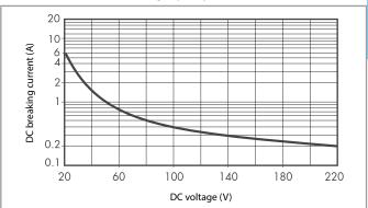
When switching a resistive load (DC1) having voltage and current values under the curve, an electrical life of ≥ 50 · 10<sup>3</sup> can be expected.
